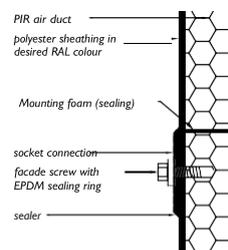
Cross-connections for hard foam ducts for outdoor installation with aluminium outer layer;
