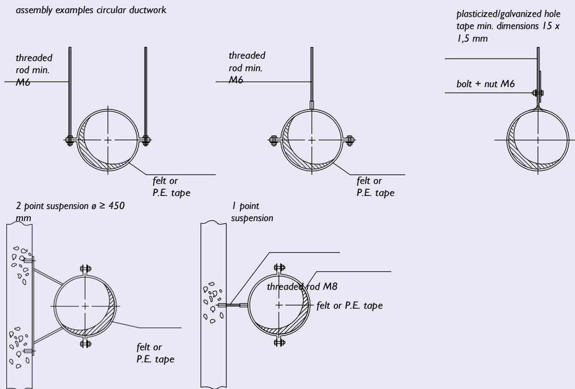
principle of suspension of uninsulated ductwork (vertical)
