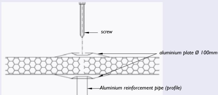
Stiffening of exterior hard foam ducts with exterior aluminium layer;
