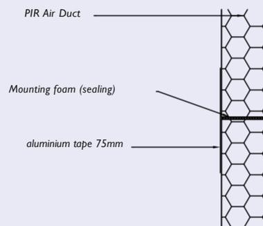
air duct connection for outdoor installation, type PUR/PIR-POL 25-30-40-50 mm
