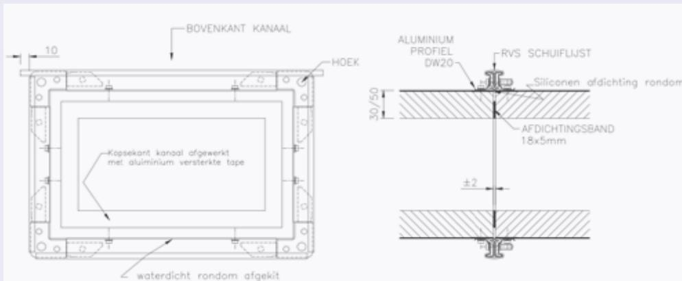
The cross-connections type DW profiles are made of aluminium, with aluminium corner pieces. The profiles are attached to each other by means of stainless steel bolts and nuts.
