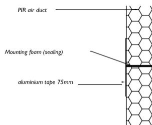
air duct connection for outdoor installation, type PUR/PIR-POL 25-30-40-50 mm
