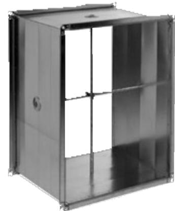
For ducts with a side  $> 800 \text{ mm}$  the previously mentioned forms of implementation apply for the duct wall surfaces concerned, whereby surfaces with a surface area of more than  $1.5 \text{ m}^2$  are additionally stiffened by subdividing them into sub-surfaces of no more than  $1 \text{ m}^2$ . This additional stiffening in the form of strips, profiles, pipes or sheets are applied internally or externally.
