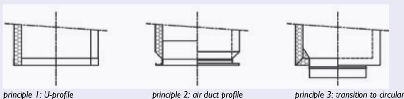
(Note: all seams in the transition must be sealed watertight in external ducts.)
