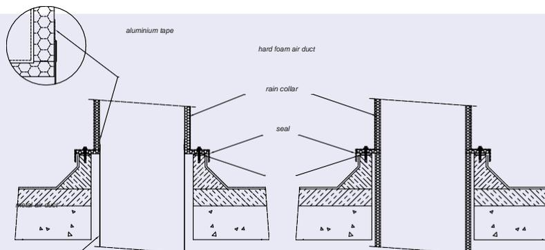
For ducts with an aluminium outer layer, a roof transit with air duct profile can also be chosen, on which the hard foam air duct directly connects. Of course, the duct (curb) must be finished weather-resistant.
