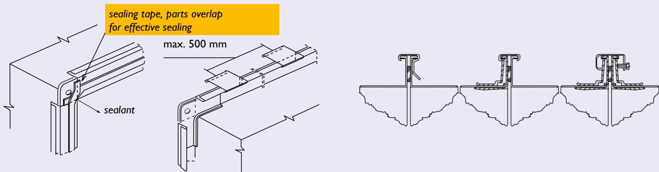
frames must have a minimum double-sided zinc layer of 140 g/m<sup>2</sup>. These cross-connections can (depending on the company) be rolled on or fixed to the duct by means of push-throughs, spot-welds, parkers or pop rivets. The cross-connections are fixed with clips, sliding strips or clamps with a maximum centre-to-centre distance of 500 mm
