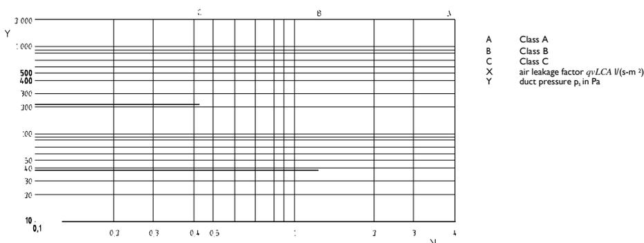
Figure taken from NEN-EN1751 (2014): graphical representation of the limiting values for airtightness classes
