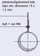
principle of suspension of uninsulated ductwork (vertical)
