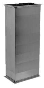
(see illustration). A closed cell sealing tape should be fitted between the cross-connections to ensure airtightness, the minimum dimension being W x H = 18 x 4 mm. All four corners are fitted with galvanised bolts and nuts, at least M 6 x 20. If sliding strips are used for the full circumference of the duct, the bolts and nuts at the corners may be omitted. Where necessary, plastic sealant will be applied internally or externally to ensure airtightness.
