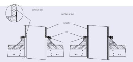
For ducts with an aluminium outer layer, a roof transit with air duct profile can also be chosen, on which the hard foam air duct directly connects. Of course, the duct (curb) must be finished weather-resistant.
