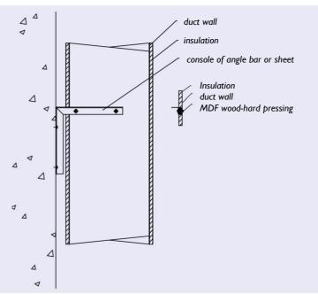
**2.10.3.3 Suspension and support for post-insolation of ducts** If the ductwork is insulated externally after installation, MDF spacer blocks 50  $\times$  50  $\times$  25 or hard pressed insulation strips 100  $\times$  25 mm must be fitted between the bottom bracket and the duct.
