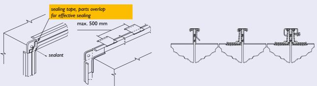
frames must have a minimum double-sided zinc layer of 140 g/m<sup>2</sup>. These crossconnections can (depending on the company) be rolled on or fixed to the duct by means of push-throughs, spot-welds, parkers or pop rivets. The crossconnections are fixed with clips, sliding strips or clamps with a maximum centre-to-centre distance of 500 mm
