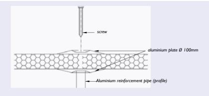
Stiffening of exterior hard foam ducts with exterior aluminium layer;
